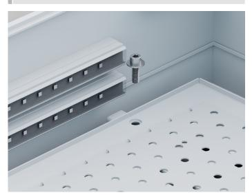
TIGHTEN DAMPER MOUNTING SCREW 🔻
