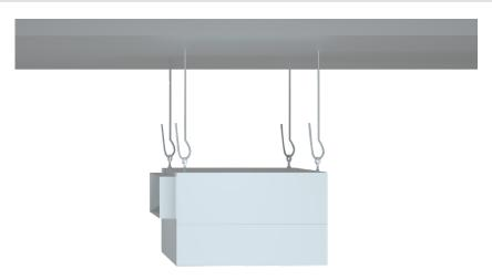
**Step 8:** Raise adjacent module assemblies, temporarily supporting the modules with hanger wire. Fasten modules together using bolts, metal washers, and lock nuts supplied by Price. Module sections will have slotted holes for fastening. Bottom of modules should be flush and level prior to fastening together.
